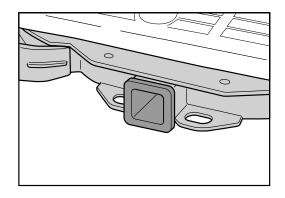
**Clamp-On Bumper Hitch** – This is a temporary hitch that clamps onto the bumper assembly.
