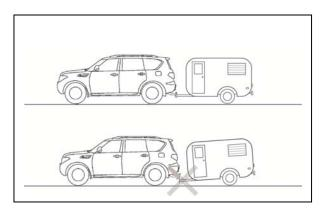
different configurations to adjust the tongue load and load transfer and hitch ball height. On some tandem axle trailers an incorrect hitch height can result in uneven trailer axle loading.
