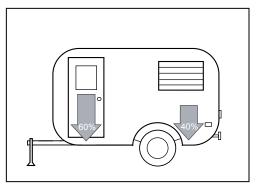
▲ WARNING-The trailer load should be balanced equally from side-to-side. Unequal side-to-side loading can negatively affect handling and braking. Once in place, all cargo should be firmly secured to prevent shifting. If the load should shift abruptly during braking or cornering, it could adversely affect the handling of your vehicle and cause a very unsafe situation and may lead to an accident or personal injury.
