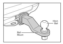
example, could result in the trailer separating from the tow vehicle. The required hitch ball size is stamped on most trailer couplers.
