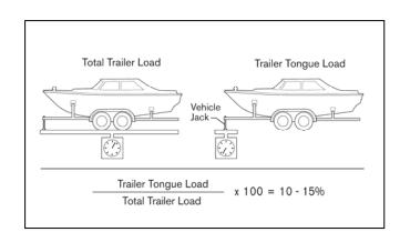
the location of the trailer jack is rearward of the trailer tongue and will not give you an accurate measurement of the true tongue load. Make sure the vehicle jack is placed directly under the trailer tongue coupler, and the tongue is set at the height/level of the tow vehicle hitch.
